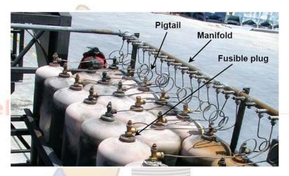
These have been involved in significant facility and motor vehicle incidents. These must be approached with extreme caution as there can be multiple cylinder failures and fire. No effective method has been developed for these incidents other than flooding quantities of water from a distance to cool and prevent more cylinders from rupturing. y Speaking
