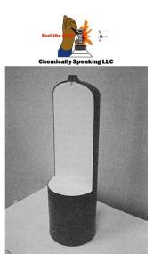
Most porous masses were previously made from asbestos since it is much more effective in controlling the decomposition due to superior physical characteristics. The porous mass is now made with a clay material with many microcavities. When a cylinder ruptures, all of the porous mass will be propelled out of the cylinder contaminating the immediate area if it contained asbestos.
