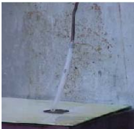
Figure 5: Vapor \text{ClF}_3 Exposure to Polyethylene Tubing, Clean and Used
