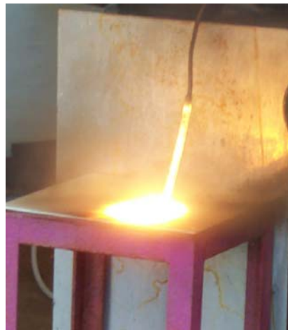
Figure 5: Vapor \text{ClF}_3 Exposure to Polyethylene Tubing, Clean and Used
