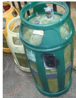
Courtesy of Nassau County Fire Academy Photo 1: The 20-pound composite cylinder was filled to its normal capacity of 80 percent with liquid propane for the tests.
