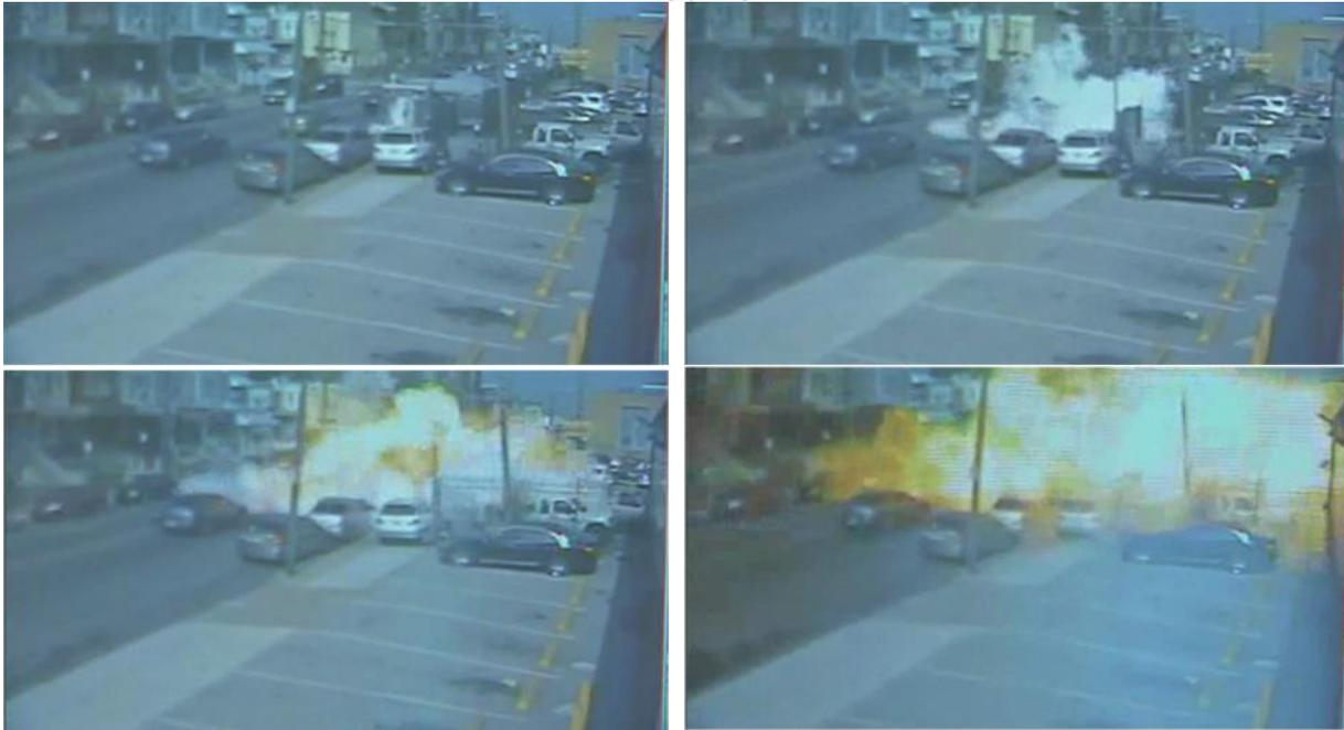
July 1, 2014 Food Truck propane cylinder rupture and deflagration in Philadelphia. The pressure relief device was illegally plugged and the cylinder was overheated by the grill that was adjacent to the storage cabinet
