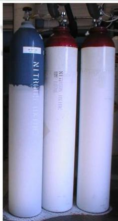
Subcooled cylinder will typically have water or ice condensed on the surface
