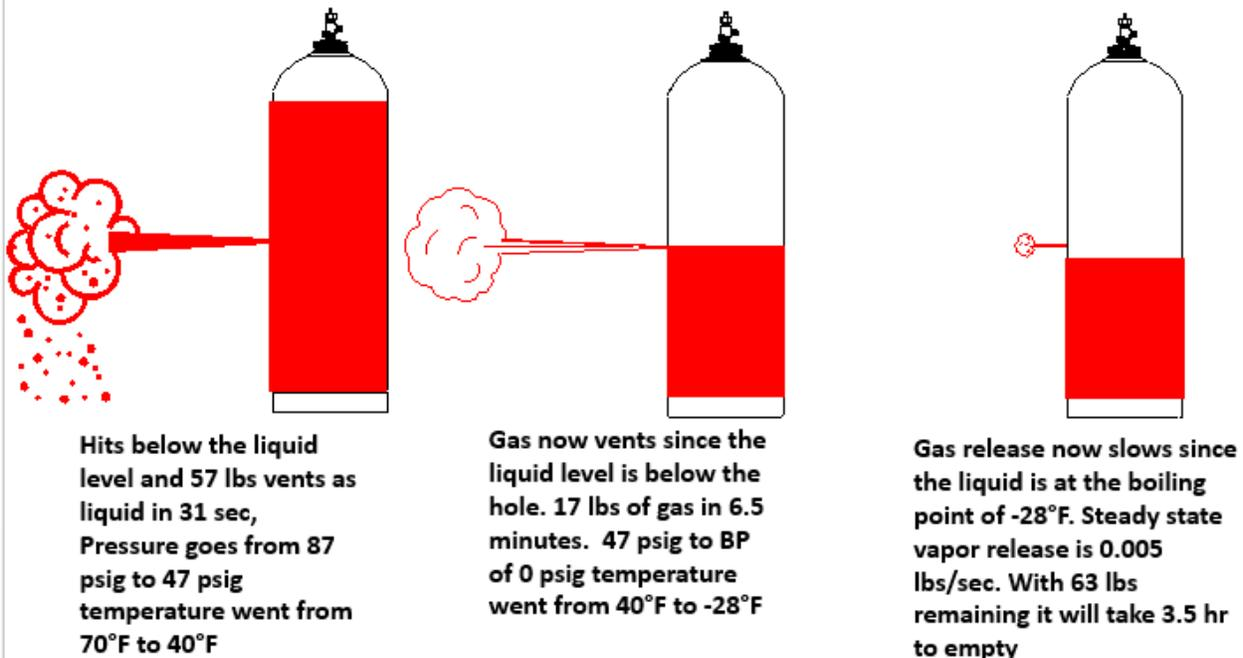
Hydrogen chloride has a critical temperature of 124.5°F (51.4°C). An HCl cylinder cooking in the sun when shot will vent its contents in minutes because it is no longer liquefied
