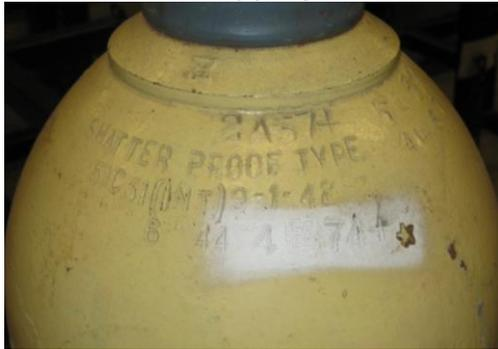
High pressure seamless cylinders (3AA) are designed to withstand bullet penetration without catastrophic failure even when pressurized to the working pressure
