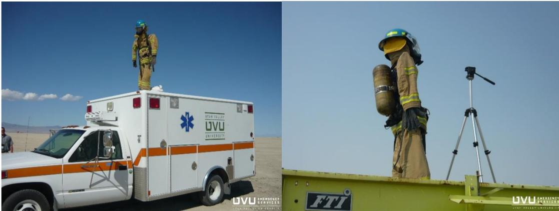
The vehicles even after 5 exposures to high  $\text{Cl}_2$  levels still ran. The turnout and SCBA were deonned and appeared to be unaffected. Concluded that a emergency responder would be protected and be able to escape a worse case  $\text{Cl}_2$  release.
