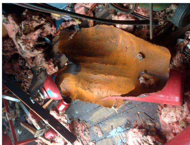
**Figure 1.** Catastrophic cylinder failure from stress-corrosion cracking.
