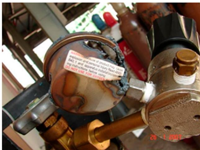
Figure 10. Regulator used for another gas service was adapted for oxygen use; it exploded when the cylinder valve was opened.
