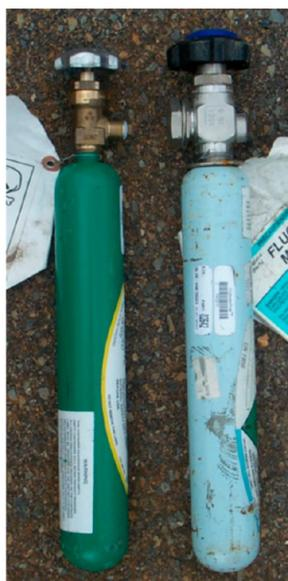
Figure 4. Lecture bottle (left) and 7X cylinder (right).
