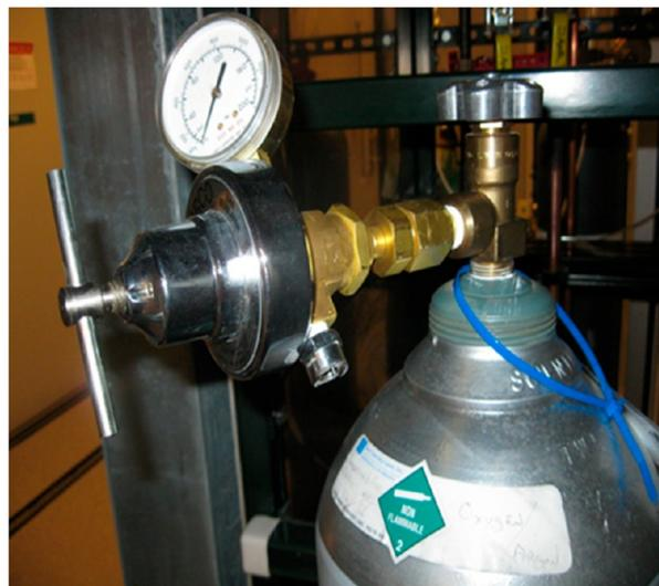
Figure 8. Single-stage regulator adapted for high pressure.
