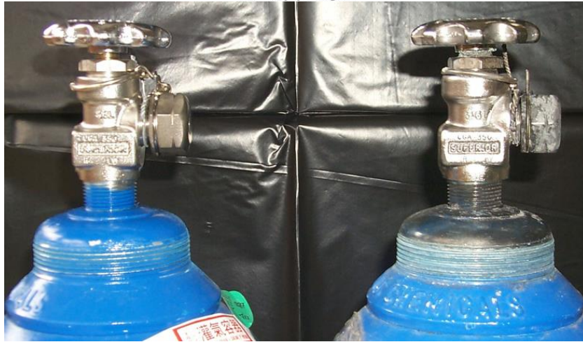
Fig 5: Clean Cylinder Left, Cylinder with PPT leak Right
