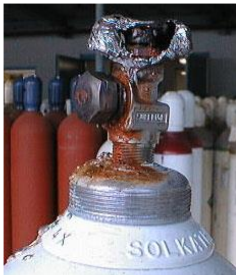
Fig 7: Phosphine Leak and Fire
