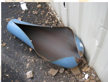
Fig. 1: Overfilled Trifluoromethane Cylinder
