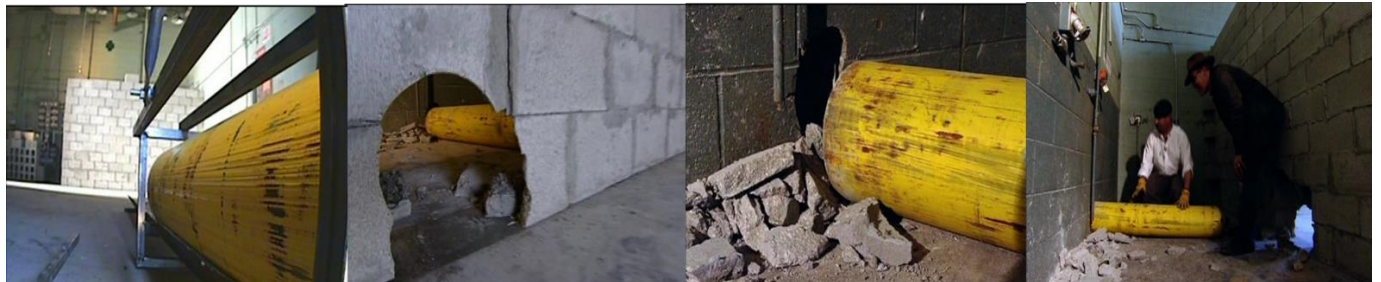
Fig 7 -10: Cylinder Impact of Concrete Block Wall
