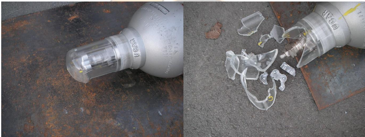
Figs 3 & 4: Polycarbonate Cylinder Cap Drop test
