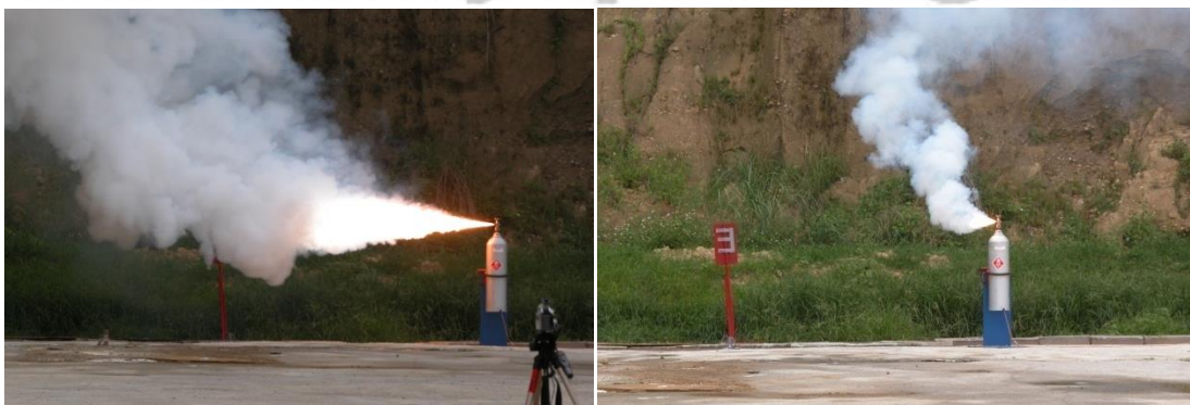
Figs. 14 & 15: Silane Flames With and Without a 0.010" (0.25 mm) RFO (1,100 psig) 23
