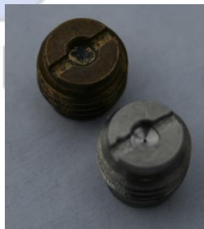
Fig. 4: Brass and Stainless Steel Superior Valve RFOs
