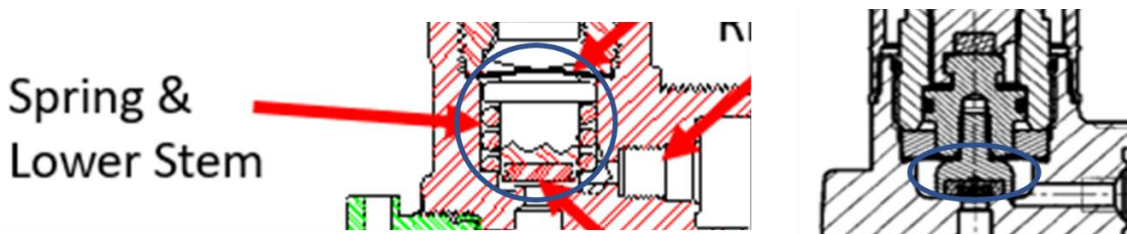
Fig. 13: Spring Loaded Diaphragm Valve and Tied Diaphragm Dead Space
