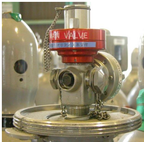
Fig. 26 & 27: Neiriki Valve Without Actuator Attached and Pneumatic Actuator
