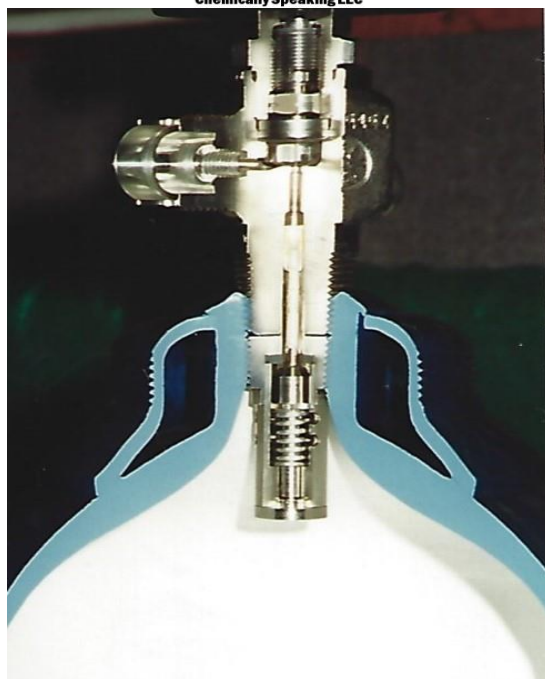
Fig. 50: Whalen Valve Cross Section
