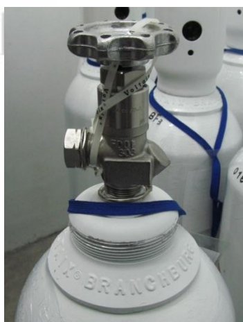
Fig. 6: Cylinder Valve Tied Closed
