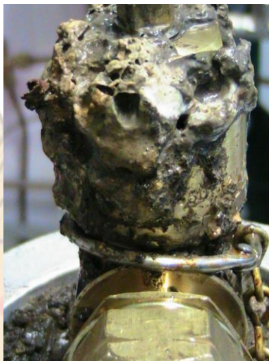
Fig 9: Melted Cylinder valve Handwheel
