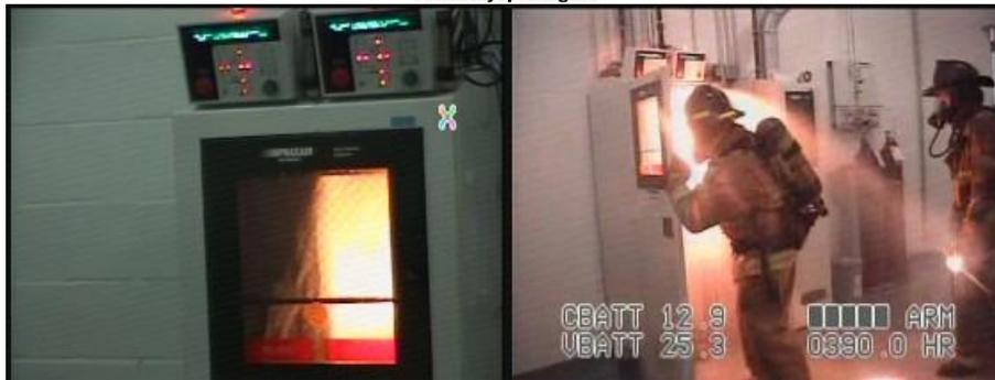
Since both cylinders of silane were made of aluminum there was concern of thermal embrittlement which can cause the cylinders to rupture. The sprinkler water cooled the cylinders preventing this from happening. The reason there is fire only on the right side is because of the metal separation plate required between aluminum cylinders of silane for the same reason.
