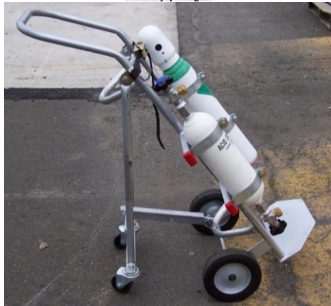
Fig.17: Leaking Cylinder Cap Cart (Photo by E. Ngai)
