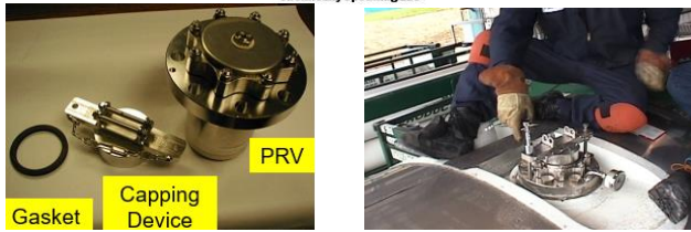
Figs. 9 & 10: Capping Device and PRV. Assembly of Capping Kit (Photos by E. Ngai)
