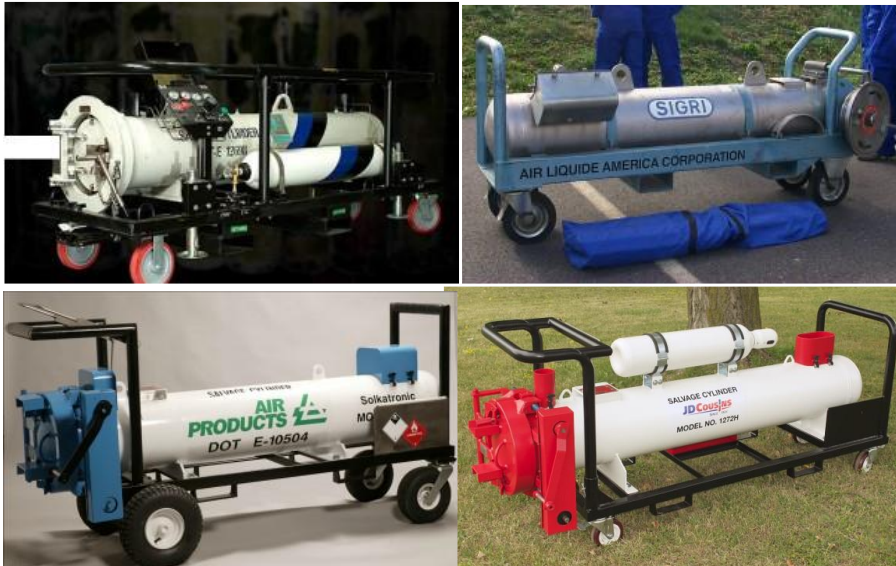
Fig. 3: ERCV's for Large High Pressure Cylinders, 50 liter or less (Photos by E. Ngai)
