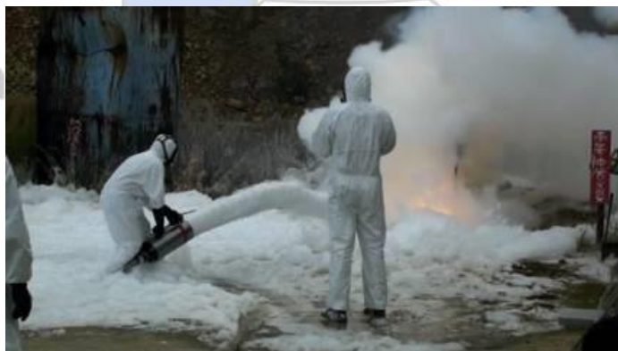
Fig. 28: Medium Expansion Foam Application onto TCS Fire (Photo by Prof J.R. Chen)
