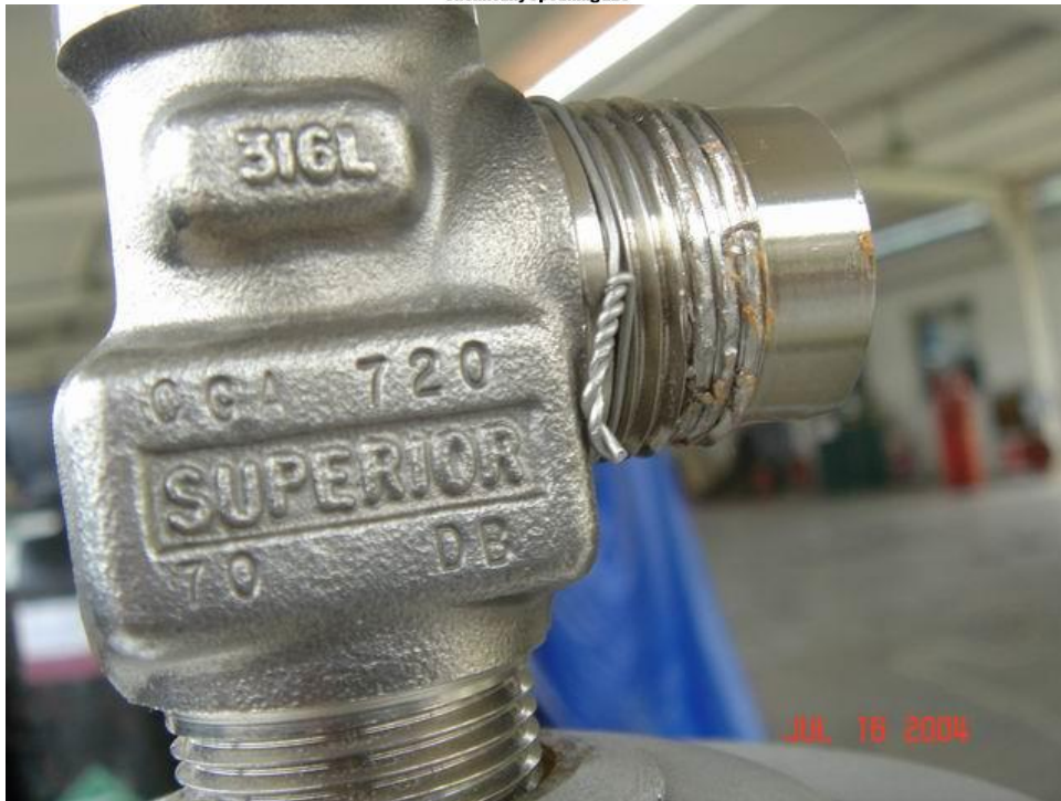
Galled threads after nut removal
