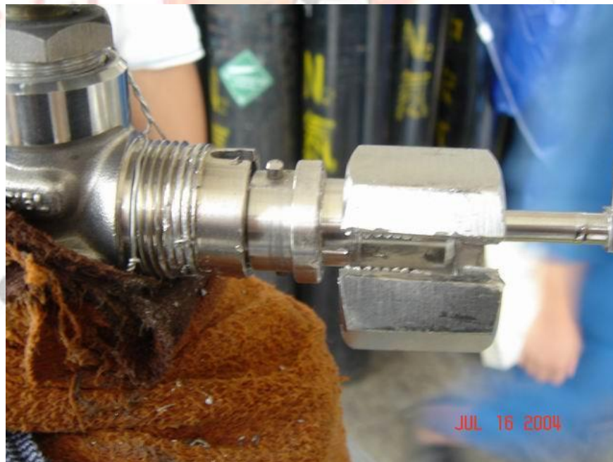
DISS Nut after splitting (NH 3 example)
