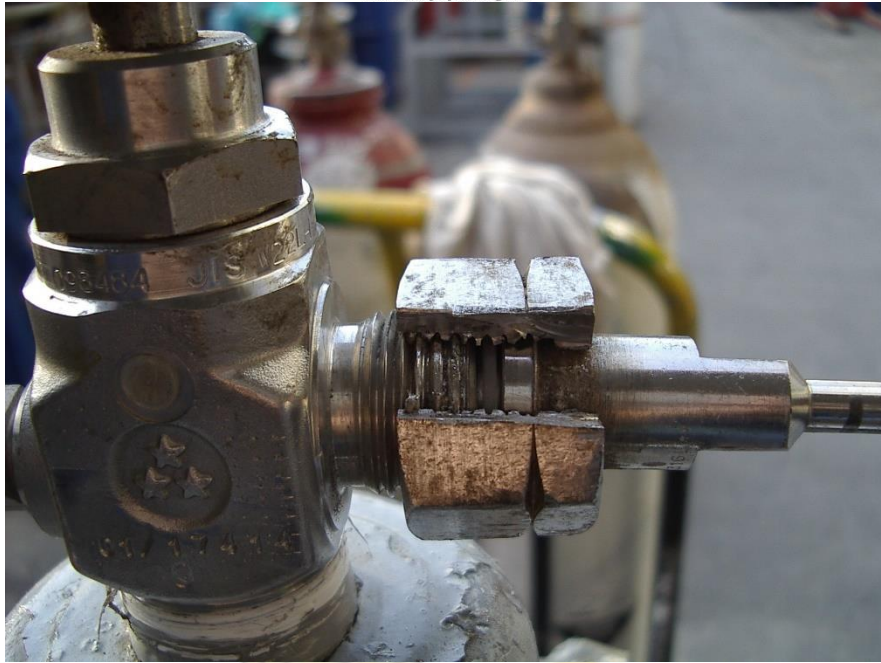
CGA Nut after splitting (Silane example)
