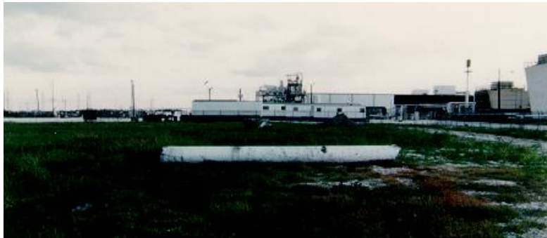
Fig. 11: Ruptured Tube Flew Over 800 ft
