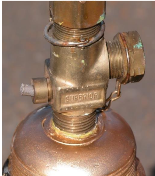
Fig. 5: Fuse Metal That Extruded Until the HCl Leaked
