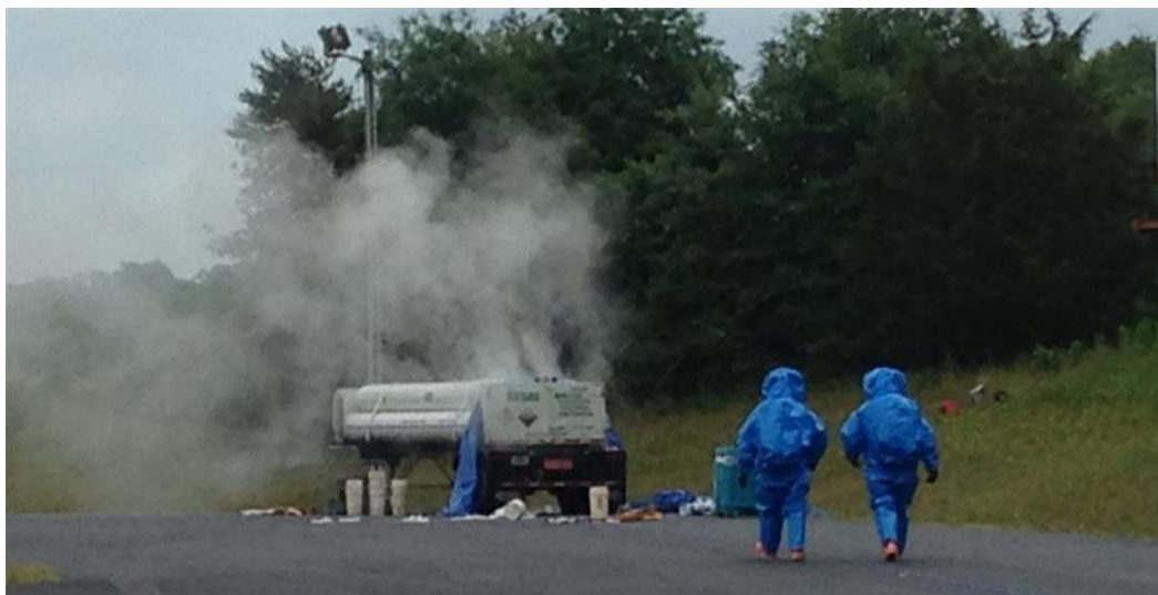
Fig. 13: Leaking Tube Trailer
