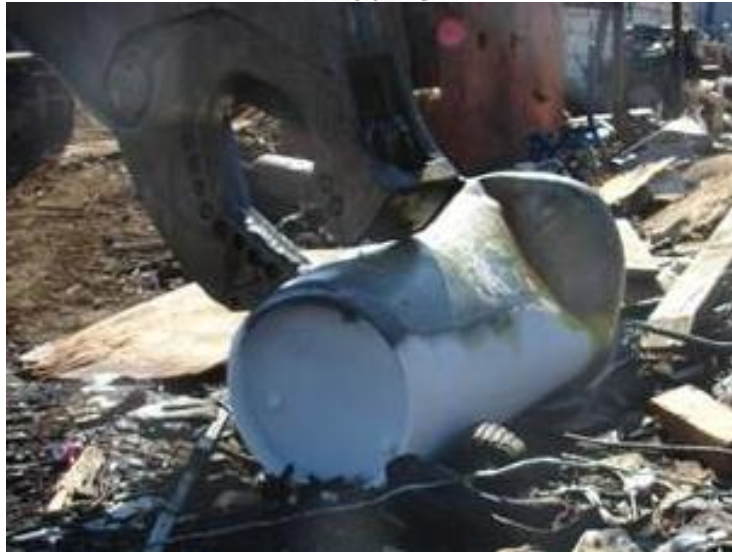
Fig 6: "Empty" chlorine ton cylinder crushed at junk yard
