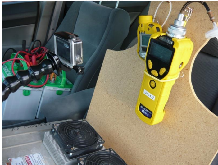
Gas Sensors in Car with Go Pro
