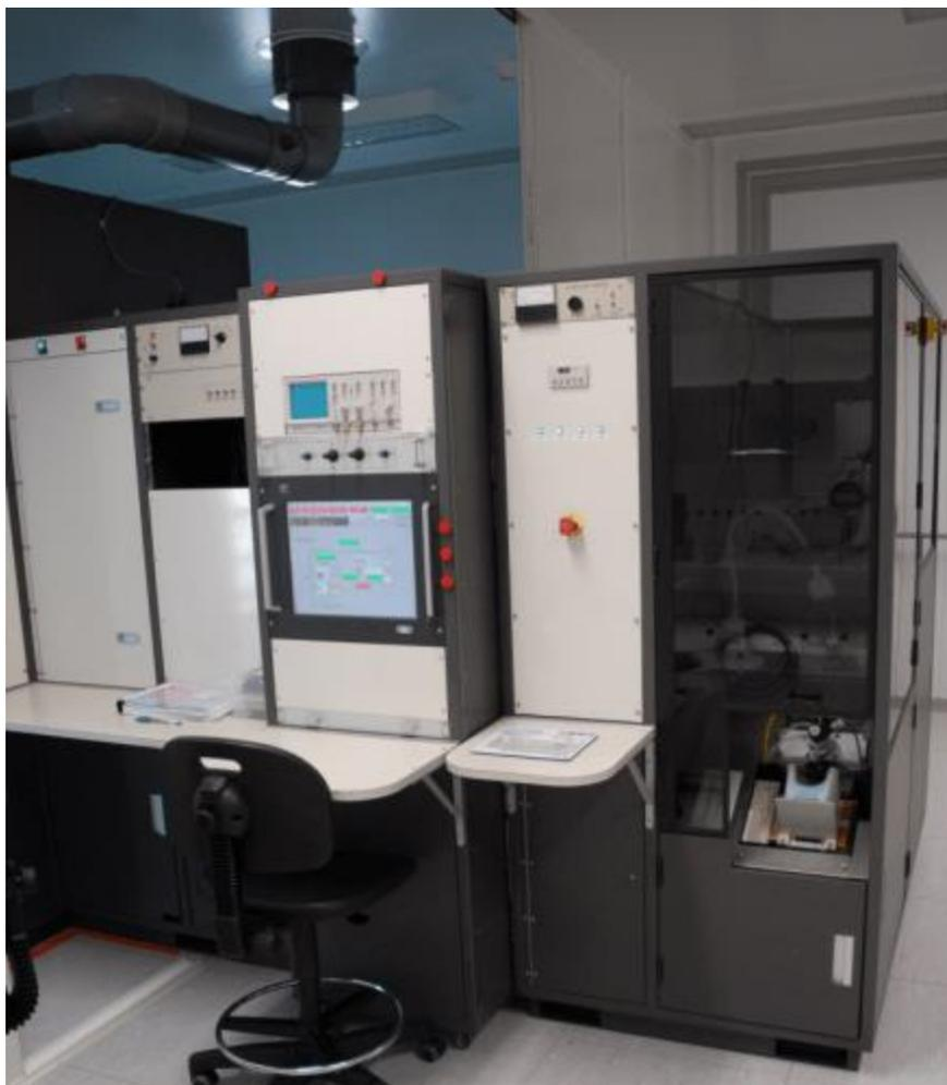
Figure 6 – Ion implanting tool – Guillaume Paumier (user:guillom), [CC BY-SA 3.0](https://creativecommons.org/licenses/by-sa/3.0/), via Wikimedia Commons
