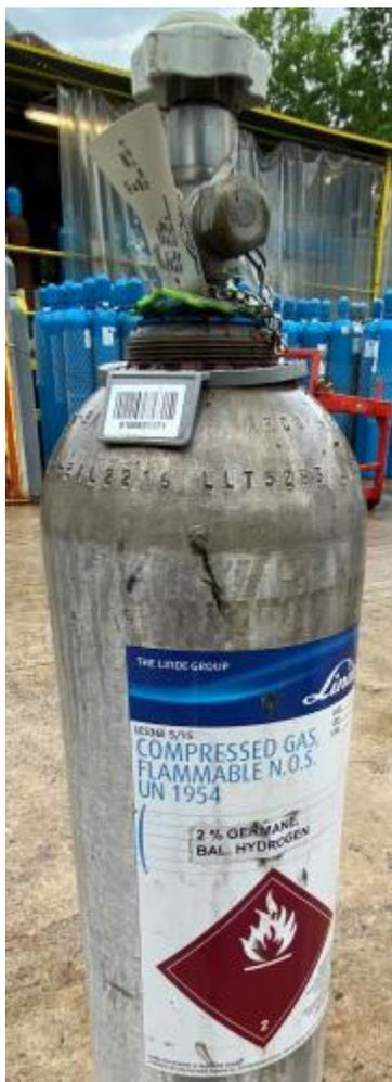
Figure 29 – Germane 2% in hydrogen cylinder.
