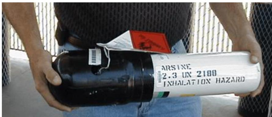
Figure 7 – Cylinder of arsine used for ion implantation.
