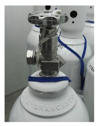
Figure 21 – Cylinder valve wired shut before dust cap screwed in place.
