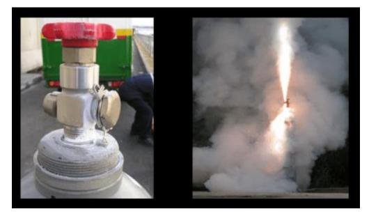
Figure 10 – Left, sand around a leaking valve on a silane cylinder. Right, spontaneous fire and formation of silicon oxides from silane release. Used with permission of Dr. Vasilis Fthenakis, Columbia University.
