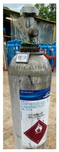
Figure 29 – Germane 2% in hydrogen cylinder.
