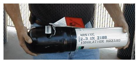
Figure 7 – Cylinder of arsine used for ion implantation.
