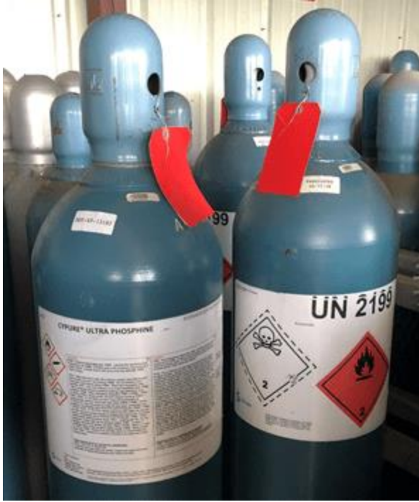
Figure 6 – Cylinders of pure phosphine for MOCVD.
