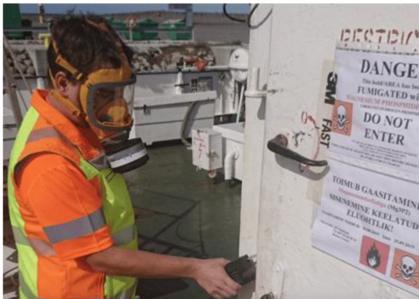
Figure 10 – Checking to be sure phosphine is not leaking from sealed ship hold containing magnesium phosphide. Photo used with permission of Fumiteam.ee.
