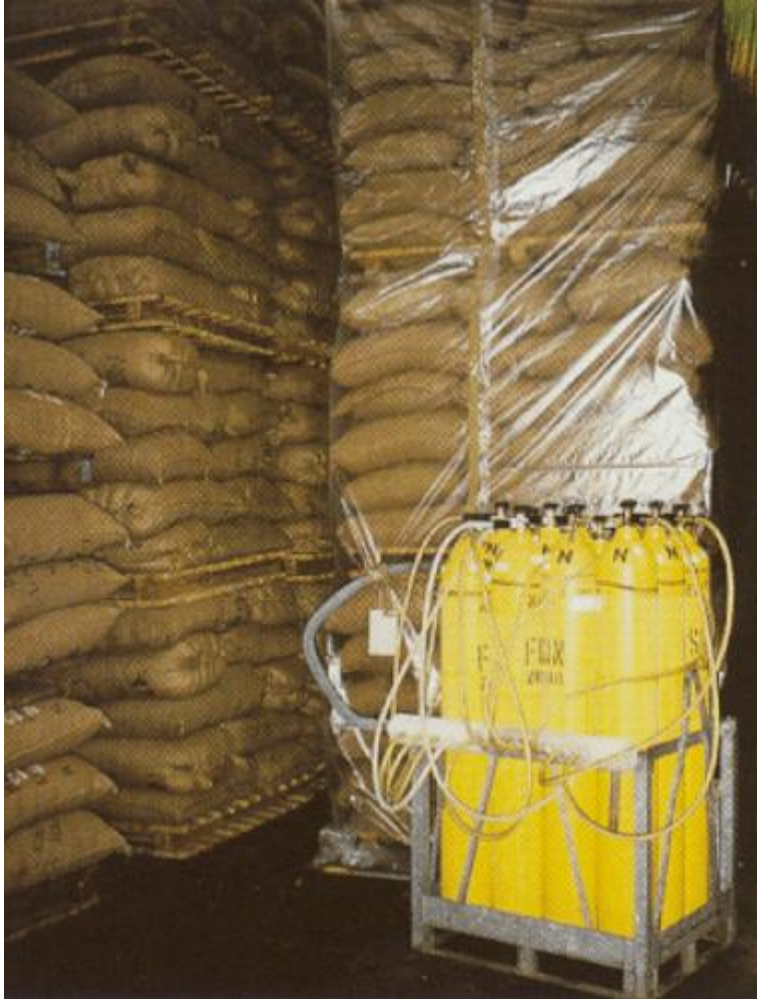
Figure 7 – Phosphine in nitrogen for grain fumigation. Photo used with permission of Messer (messer-us.com).
