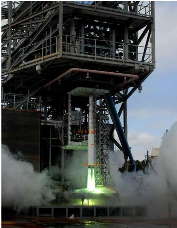
Figure 4 – Ignition with triethylaluminum/triethylboron https://www.nasa.gov/exploration/systems/sls/sls-acoustic-testing-2014.html
