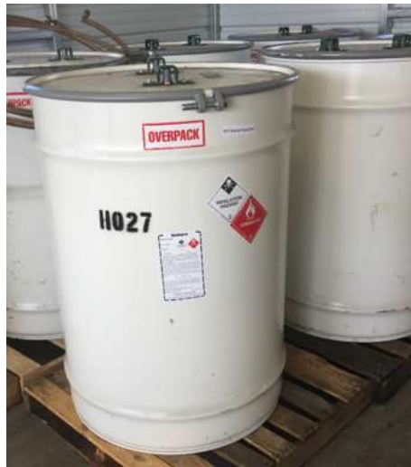
Figure 17 – insulated drum containing dry ice and diborane cylinder
