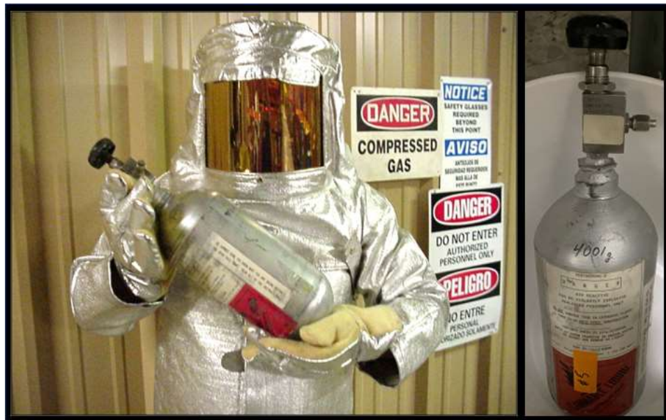
Figure 15 – Pentaborane cylinders pressurized with nitrogen
