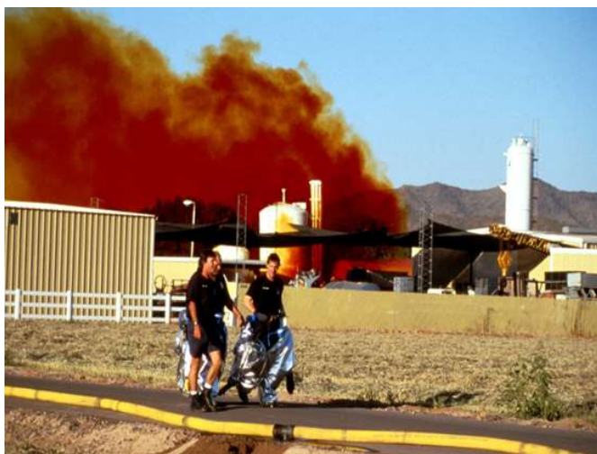
Figure 12 – NO 2 formed from spill of concentrated HNO 3
