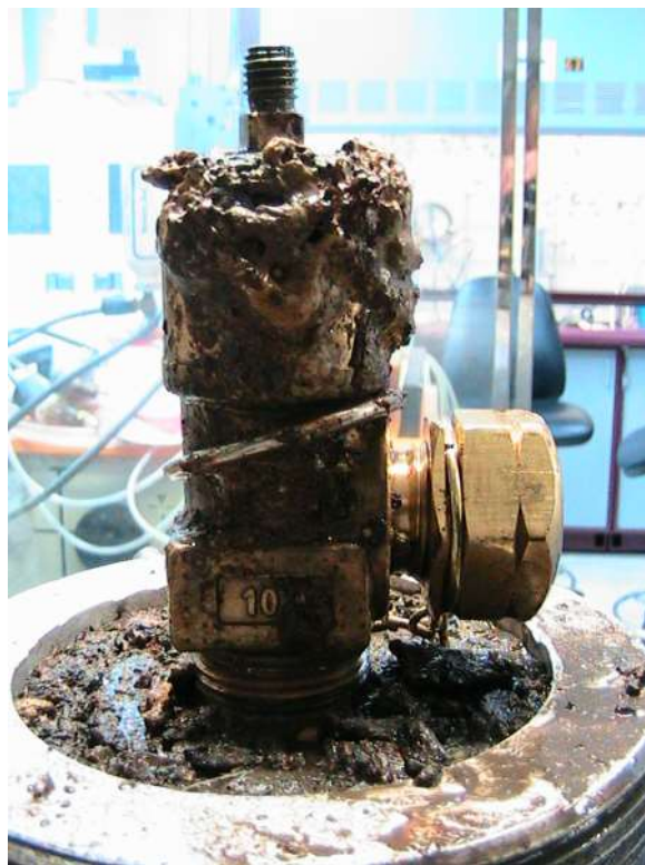
Figure 9 – Melted valve on a cylinder of diborane after
